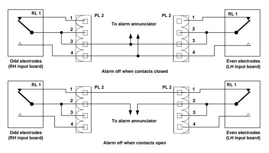
(Switch SW5 is set to ES for low level alarms and set to EW for high level alarms)
